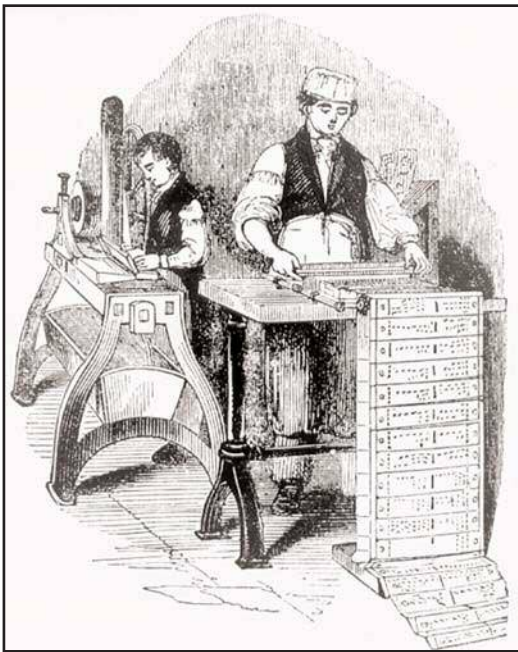
Figure 5. Workers making Jacquard punched cards. Kopplin: "An Illustrated History of Computers," Internet
