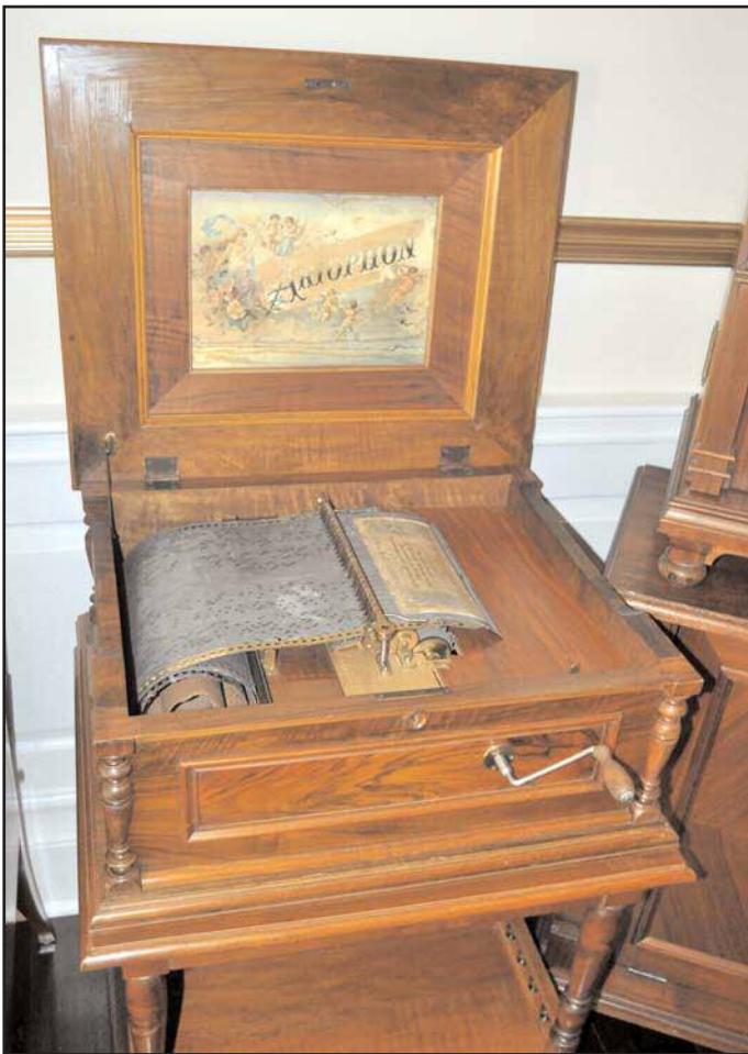
Figure 7. An existing Ariophon , this one using a coiled zinc sheet. The folded books would have sat in the depression on the left side of the case.
