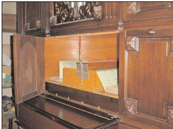
Figure 68. Upon opening the doors above the keyboard the keyframe and book can be seen.
