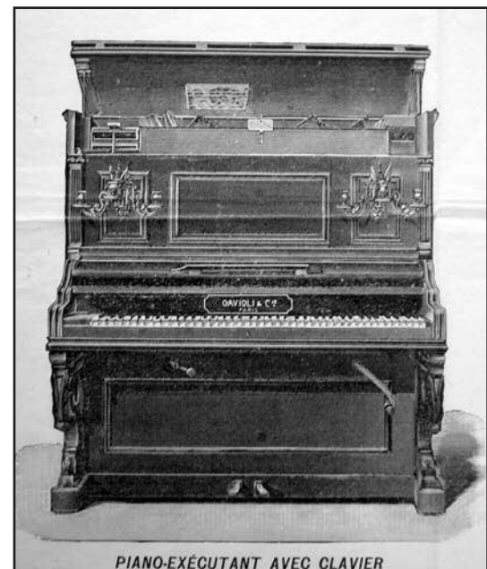
Figure 48. The Piano Exécuteur with its book-playing mechanism located at the top of the piano.
